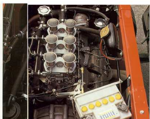
Below: The engine chosen for the Stratos was the 2418-cc iron-blocked built development of the two-litre aluminium Ferrari quad-cam V6 originally designed for Formula 2 racing and then used in the Dino 206. In standard form it had two valves per cylinder and breathed through three 24mm 40-mm twin-choke Weber carburetors. It was used both in Ferrari's 2400 series and in Fiat's own Dino, but by the time the Stratos was homologated in 1974, neither was in production.
