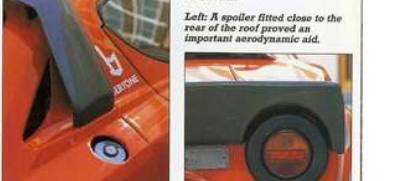
Left: A spoiler fitted close to the rear of the roof proved an important aerodynamic aid.
